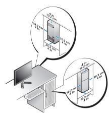
If your computer is installed in a corner on a desk or under a desk, leave at least 5.1-cm (2-inch) clearance from the back of the computer to the wall to permit the airflow required for proper ventilation.
